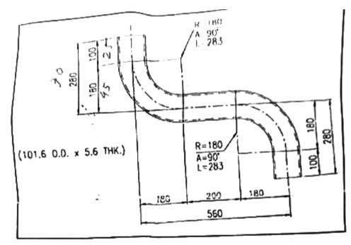
Bend as shown in the figure.(Use the scale of 1:4).
